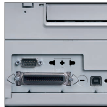
RS 232, IEEE 1284 AND USB 2.0 INTERFACES plus expansion slot
